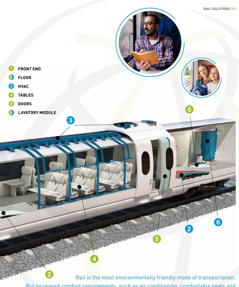
But increased comfort requirements, such as air conditioning, comfortable seats and tables, easily accessible lavatories and CET tanks have made trains heavier and more expensive to operate. To maintain its environmental advantage, energy efficiency has to be improved – without compromising passenger safety and comfort.
